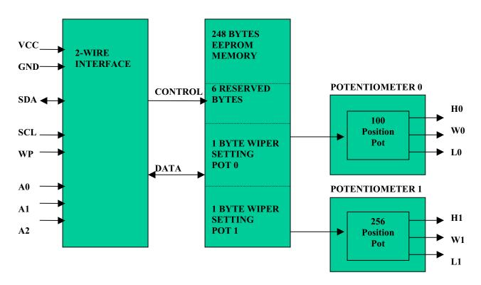
Up to eight DS1845s can be installed on a single 2-wire bus. Access to an individual device is achieved by using a device address that is determined by the logic levels of address pins A0 though A2. Additionally, the DS1845 will operate from 3 volt or 5 volt supplies. Three package options are available: Flip Chip Package, 16-ball STPBGA and 14-pin TSSOP.
